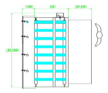
1, the machine in accordance with the requirements for installation location plan in place. And then adjust the machine level level error is not more than + / - 1.5 mm
