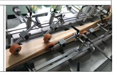
Template fixing lever Adjust the position of the left and right of the template Nsert wheel adjustment seat Adjust the width of the side of the paper bag Traction cylinder, using Taiwan's AirTAC brand, the drawing material is more flat, the pressure is even, and the effect is more ideal.
