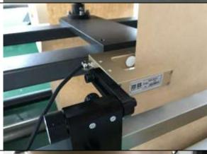
Using the German (sick) color photoelectric tracking, precise tracking of paper printing photo, automatic alignment, if change the paper roll, power does not need to adjust the cutting position. Automatic stop if color error ,reduce Scrap rate.
