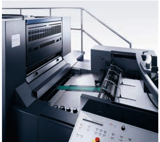
Optimum sheet transport – the feeder with central suction tape.
